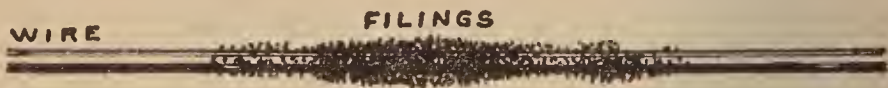
FIG. 1.—If a current of electricity is passed through a wire, the wire will attract to itself iron filings.
